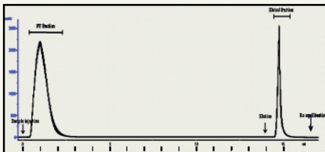
Fig. 1. Overlay of chromatograms of run number 1, 50 and 300 of repeated affinity removal of IgG. The overlay proves that the depletion procedure can be reproducibly repeated at least 300 times without loss of binding capacity.
